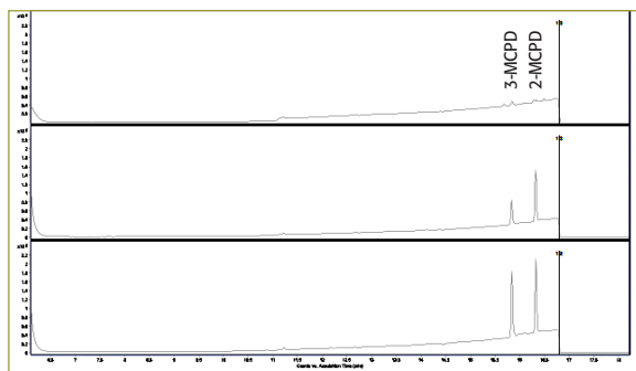
SIM chromatogram m/z 198 : Top: Virgin olive oil used as blank oil. Middle: Edible oil sample assay B (3-MCPD). Bottom: Edible oil sample assay A (3-MCPD + glycidol).
